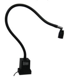
LED lamp made up of aluminum and ABS spot, n.1 power LED sources, adjustable lens, stainless-steel gooseneck arm covered by PVC, ABS base with fastening holes and on/off switch. Built-in LED driver. Power supply 230V 50/60Hz. Current 700mA.
